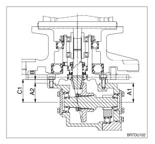
(4) On the adjusting the tooth contact of spiral bevel gear, if changing the shim, idle of decrease the shim inserting between the cover of shaft both side and the gear case shim thickness.
